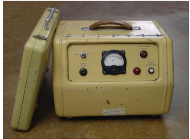
Figure 5. The first DC defibrillator ID-1-VEI for external transthoracic and internal use made in the USSR in 1952. Paddles and cords were stored in the separate metal box, which is leaning on the device. The defibrillator in this picture was given in 1958 to Dr Robert Hosler, an associate of Dr Claude Beck, by Dr Vladimir Negovsky in Moscow during Dr Hosler's visit to Russia. Courtesy of the Dittrick Medical History Center, Case Western Reserve University, Cleveland, Ohio.
