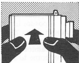
Set the camera for rewind by depressing the rewind release button in the base (*top, left*). Unfold the rewind crank and rewind the film (*top, centre*). Open the camera back and pull up the rewind knob (*top, right*). Remove the cassette (*bottom, left*) and close the camera back (*bottom, right*).
