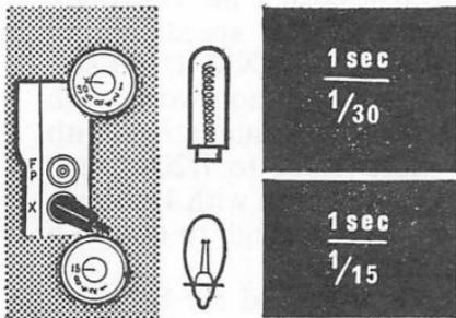
The Minolta SR (except T303 and X series) carries two flash sockets. When the plug from the flash gun is fitted in the top socket, marked FP, the camera is synchronized for focal plane-type flash bulbs at all shutter speeds to 1/500 second (or up to 1/100 second on SR-7 and T101).
