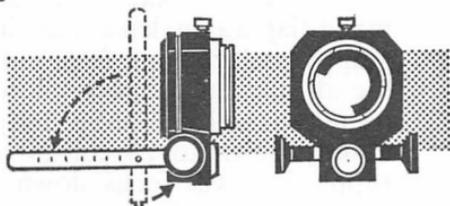
The extension bellows De Luxe gives magnifications (with the 55 mm. lens) up to 3.2 and focuses down to about 1 1/4 in. The bellows is shown here with the bellows lens hood and transparency copier (see page 58).
