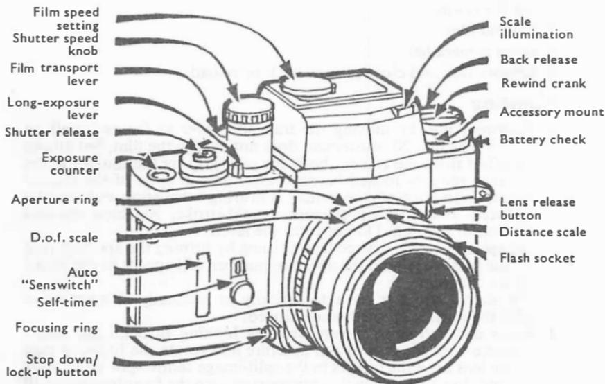
The Minolta XM uses sophisticated circuitry for fully automatic operation with a replacement prism unit. The "Senswitch" on the camera front operates the metering system as the camera is gripped normally. Four replacement finder units are available and nine focusing screens.
