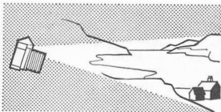
To take general reflected light readings with the Minolta meter, either point it directly at the subject or, with outdoor views, direct it slightly downwards to cut down the amount of light reaching it from the sky.
