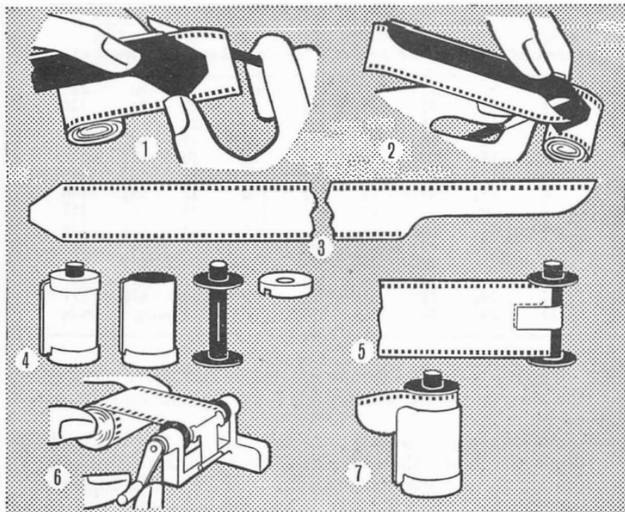
1. The correct trimming of the wedge-shaped end (which is attached to the centre spool of the cassette) with standard trimming template.
