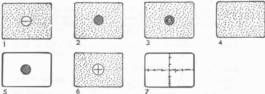
The focusing screens are: 1, Matt fresnel field with split-image rangefinder. 2, Matt fresnel field with microprism rangefinder. 3, Matt fresnel field with both rangefinders. 4, Matt fresnel field only. 5, Clear fresnel with microprism rangefinder for various lenses (three types). 6, Matt fresnel with crossed hairs on clear field. 7, Clear fresnel with graduated cross lines.
