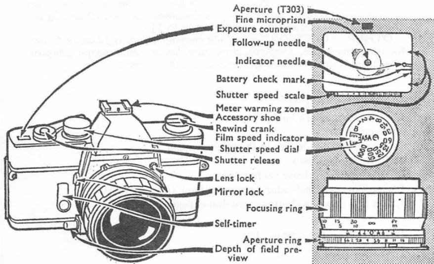
The film transport lever operates the exposure counter as well as tensioning the shutter. Light reaches the meter cell through the camera lens and causes the indicator needle in the viewfinder to move. A follow-up needle is connected to aperture, film speed and shutter speed settings. A mirror lock is fitted so that mirror can be held up when
