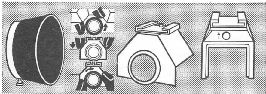
The Minolta SR lenses accept push-on hoods (*left*). Lenses of 100 mm. and up are supplied with hoods. The accessory shoe (*centre*) can be fitted to the SR cameras after turning the viewfinder eyepiece ring clockwise and removing it. Then replace the eyepiece ring to hold the accessory shoe in place. The accessory shoe for the V model clips into the grooves of the eyepiece.
