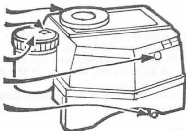
Match-needle TTL finder displaying shutter speed and aperture
