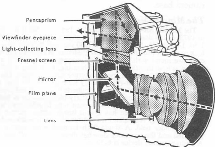
Above: A section through the camera shows the optical system of lens, mirror, viewfinder lens and fresnel screen, pentaprism and viewfinder eyepiece. The broken line indicates the path of the light when the mirror is in position for viewing and focusing.
