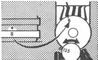
Using the Minolta SR Meter. *Left to right, top:* Attach the meter to the camera. Set the film speed. Pre-select the shutter speed. Set scale selector dial according to light conditions. *Left to right, bottom:* Point camera towards subject. Read off the aperture required and set it on the lens. Alternatively, the aperture can first be set on the lens and the shutter dial rotated until the meter needle points to that aperture.
