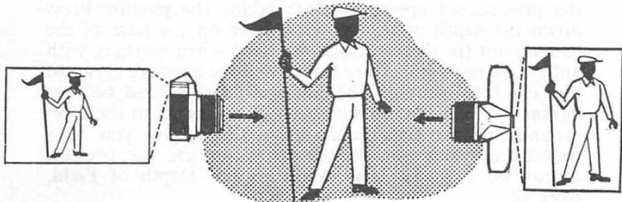
certain point, beyond which it will again lose definition. At this "beyond" stage turn the mount back again, narrowing down the degree of movement until you arrive at the point of best definition. The centre of the reflex image is a microprism area; in it you will see the image snap into critical focus. Earlier models had clear glass centres.
