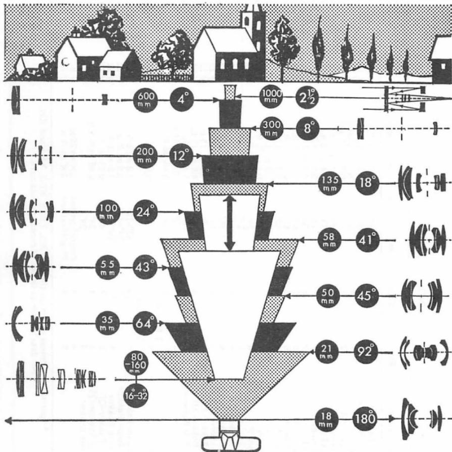
Lenses of many different focal lengths are available for the Minolta SR. They range from 1.5° to 180° angle, i.e. 1600 mm. to 18 mm. focal length. The longer the focal length, the larger the image scale, but the smaller the view covered. The shorter the focal length, the wider the view but the smaller the scale of the image.
