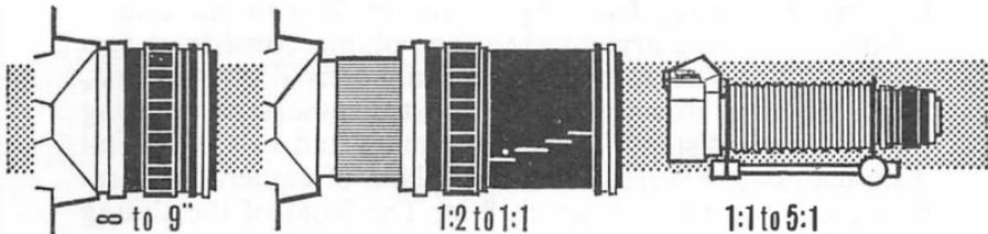
The Macro Rokkor lens (left) focuses from Infinity to 9 in. Used with an extension tube (centre) it gives 1 : 2 to 1 : 1 reproduction ratios. With bellows extension (right) it can give reproduction ratios from 1 : 1 to 5 : 1.
