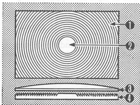
The Minolta SR screen consists of a light-collecting lens (3) over a fresnel screen (1). The fine lines of the screen (1) present a bright image right out to the corners. The central portion of the screen (2) consists of microprisms for critical focusing. In the SR models, this area is clear.
