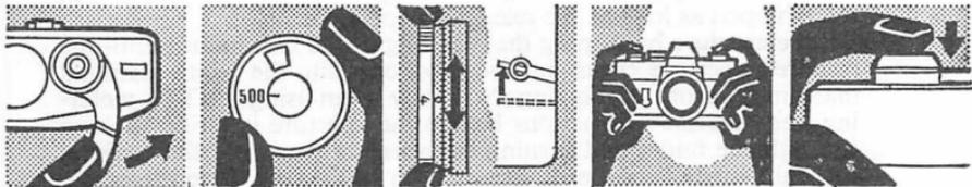
Shooting with the Minolta SR-T101. From left to right: Advance the film and tension the shutter with the film transport lever. Set the shutter speed required and line up the follow pointer by adjusting the aperture. Focus and compose the picture and press the shutter release gently.
