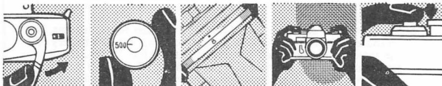
Shooting with the Minolta SR-I, SR-I (V) and SR-IS. From left to right: Advance the film and tension the shutter with the film transport lever. Set shutter speed. Set aperture. Focus and compose the picture in the viewfinder. Press the shutter release gently.
