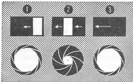
The pre-set aperture works differently. 1. Pre-select the aperture with the front aperture ring and open the iris fully with the rear aperture ring. 2. Immediately before the exposure, close down the iris to its pre-set aperture by turning the rear ring in the opposite direction. 3. Press the shutter release to take the picture.
