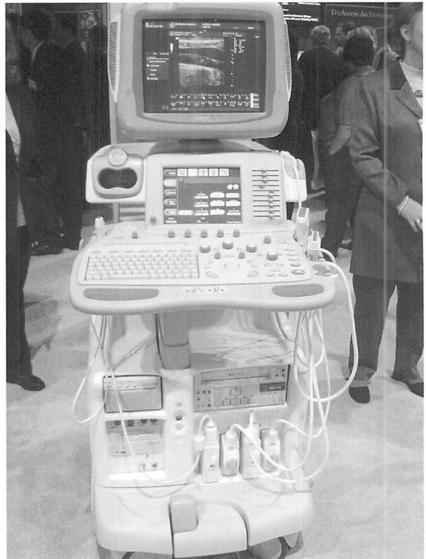
**Figure 3.1** The basic components of an ultrasound machine are the monitor, the computer, and the probes.
