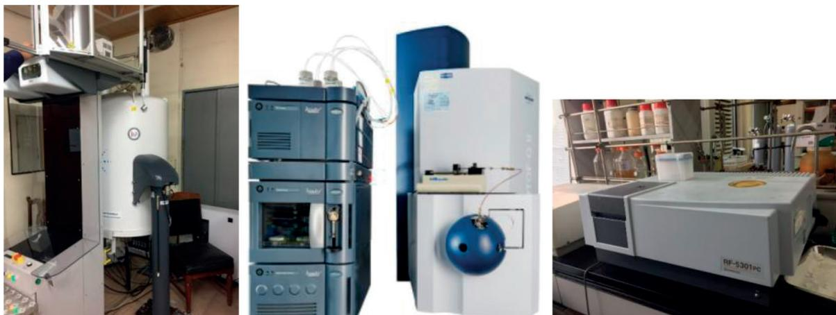
**Figure 2.** Instruments used in the scientific laboratory such as the multinuclear NMR spectrometer (left), high-resolution mass spectrometer (middle), and fluorimeter (right). (Photos acquired at KAIST (Daejeon, Korea); high-resolution mass spectrometer photo taken from [kara.kaist.ac.kr](http://kara.kaist.ac.kr)).
