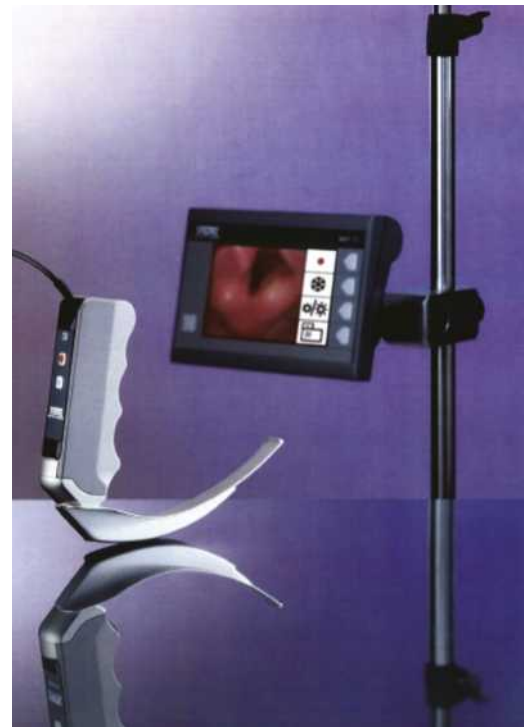
Fig. 1.13 The C-MAC videolaryngoscope (Karl Storz Endoscopy, Tuttlingen, Germany) uses an integrated complementary metal oxide semiconductor (CMOS) video chip to capture a video image from near the distal tip of an otherwise conventional laryngoscope blade. The image is conveyed to a video screen, where it is viewed by the intubator. (Modified from Brown III CA, Mick NM, Sakles JC, editors. The Walls Manual of Emergency Airway Management . 5th ed. Philadelphia: Wolters Kluwer; 2018.)
