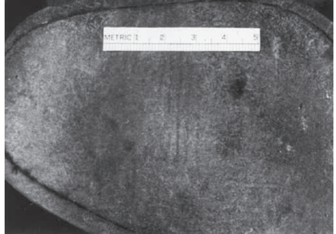
Fig. e11.28 Imprint of a brake pedal on a leather-soled shoe. This information will assist in determining the occupant's role and whether the patient's foot was on the brake or accelerator pedal at the moment of impact.
