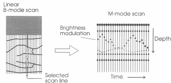
**Figure 13.8.** *M-mode scan display. Echo brightness (or grey level) indicates echo amplitude. The vertical co-ordinate represents range (depth) while the horizontal co-ordinate represents time.*
