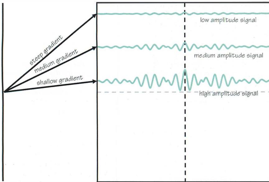
Figure 33.1 Phase gradient amplitude vs signal amplitude.
