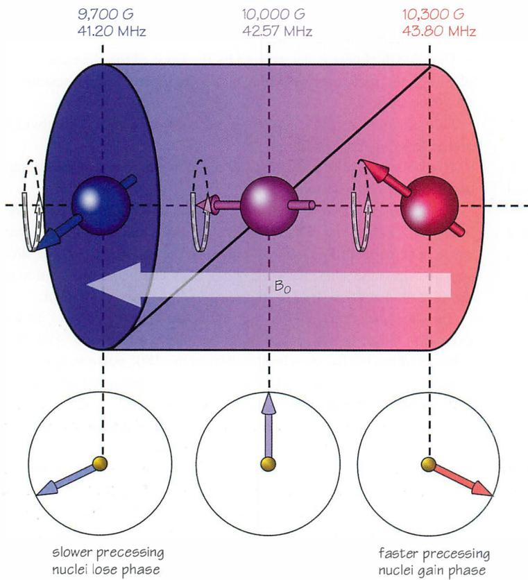
Figure 29.1 Phase encoding.
