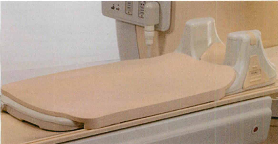
Figure 57.1 Spinal phased array coil.
