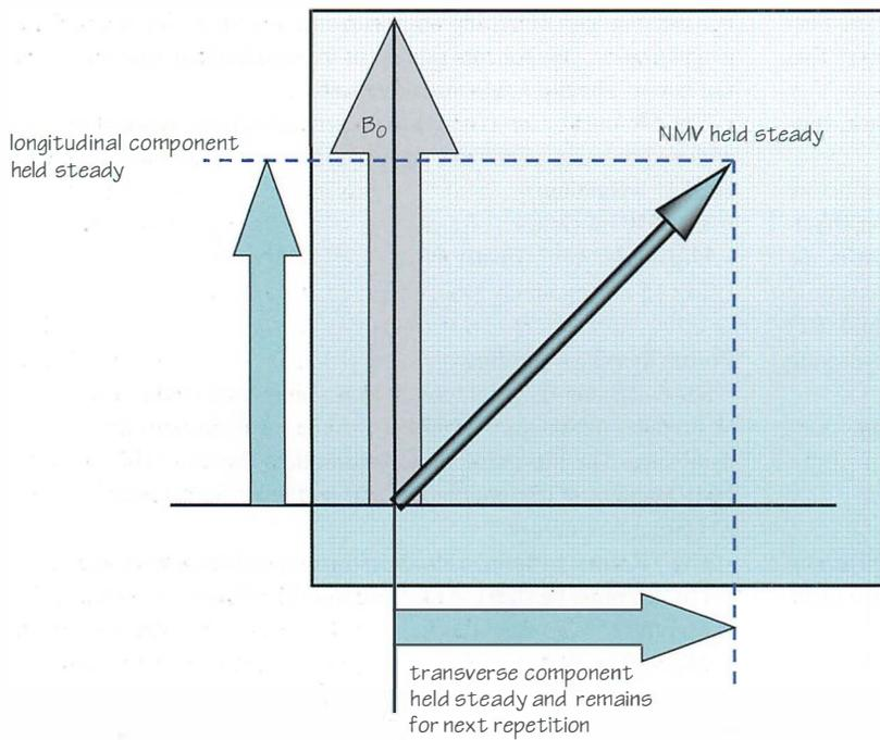
Figure 19.1 The steady state.
