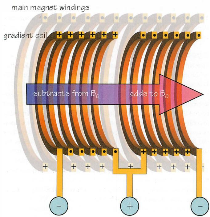
Figure 27.1 A gradient coil.
