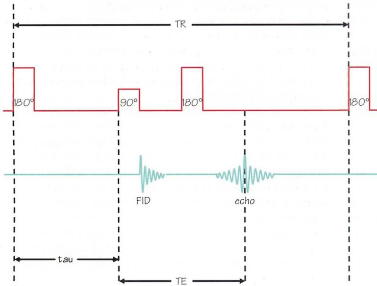
Figure 16.1 The inversion recovery sequence.
