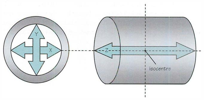
Figure 27.4 Gradient axes.
