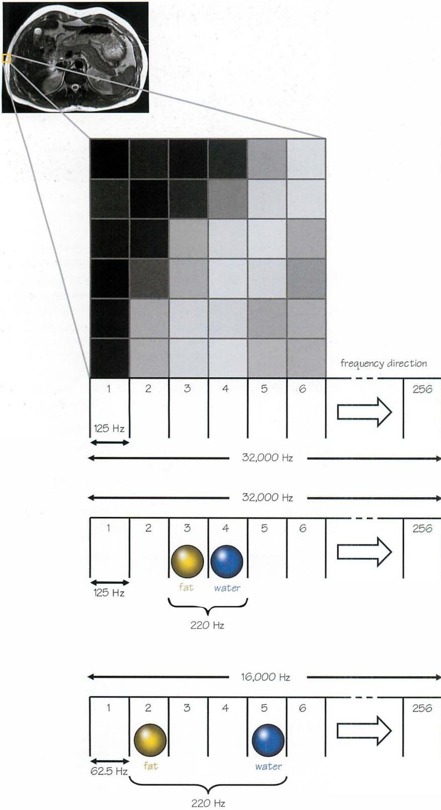
Figure 45.1 Chemical shift and the receive bandwidth.
