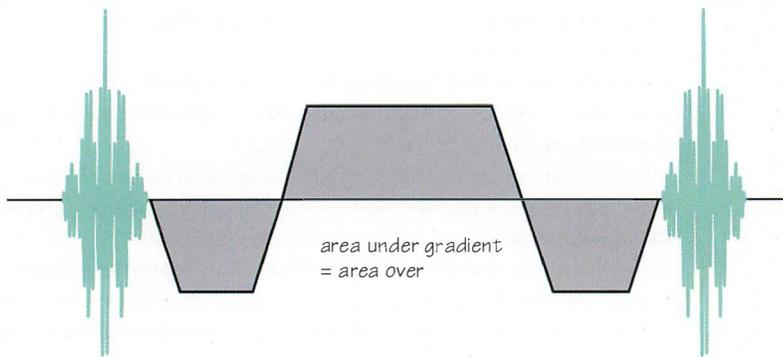
Figure 23.1 Balanced gradient scheme in balanced gradient echo.
