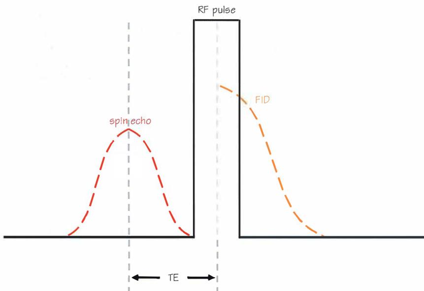
Figure 22.2 Echo generation in SSFP.
