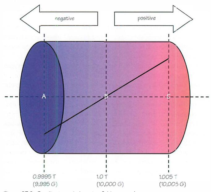
Figure 27.2 Gradients and changing field strength.
