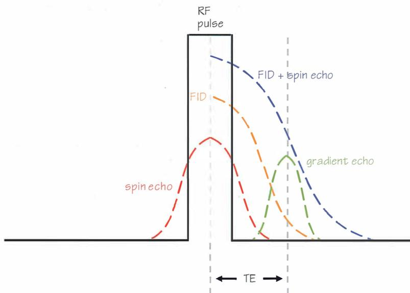
Figure 20.2 Echo generation in coherent gradient echo.
