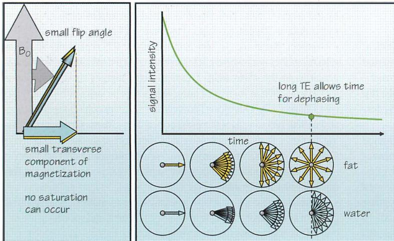
Figure 18.3 T2\* weighting in gradient echo.
