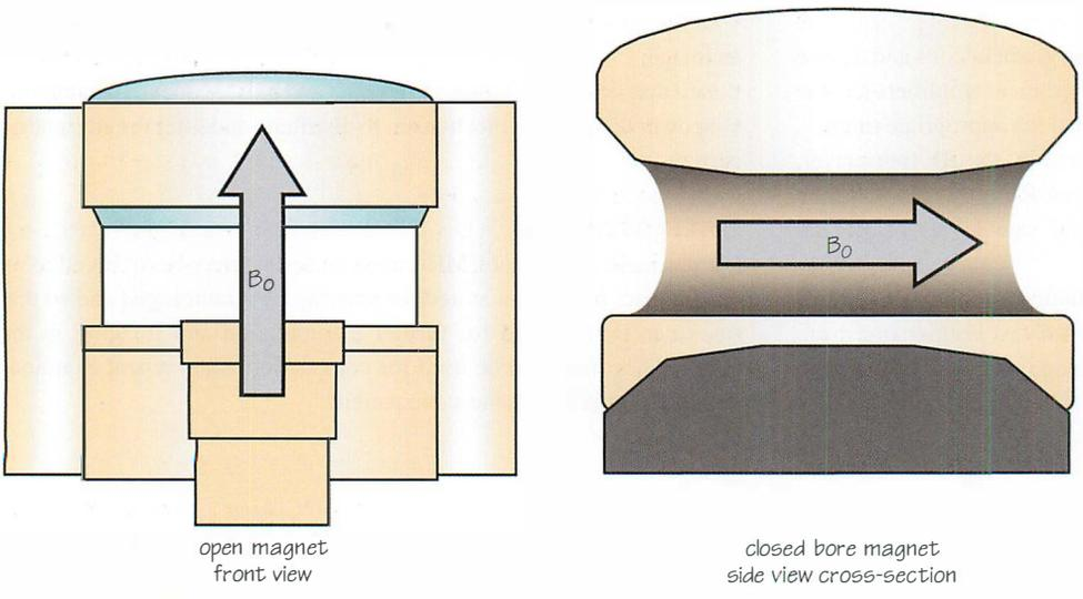
Figure 59.1 Static field in permanent and superconducting systems.
