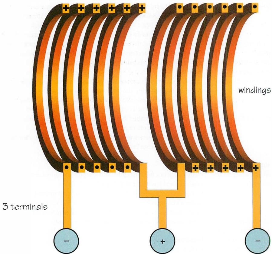
Figure 56.1 A three-terminal electromagnet used in gradient coils.
