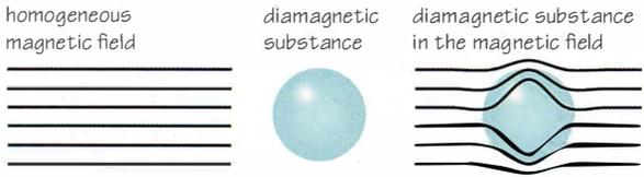
Figure 1.2 Diamagnetic properties.
