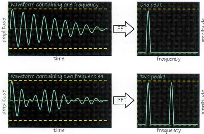
Figure 31.2 Fast Fourier transform.
