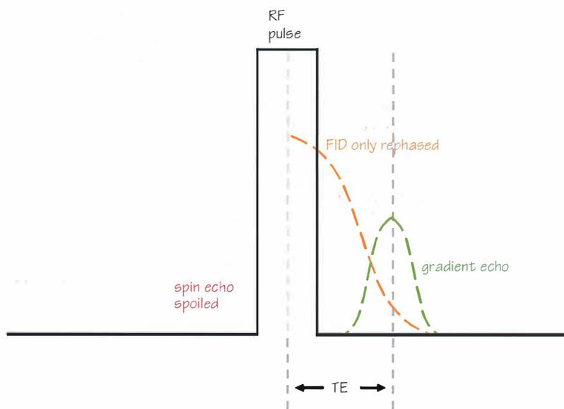
Figure 21.2 Echo generation in incoherent gradient echo.
