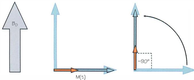
Figure 15.3 The fast recovery or 'drive' sequence.
