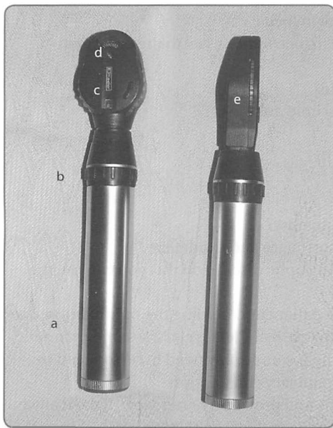
Figure 6.17.1 Parts of the ophthalmoscope. (a) handle and battery case (b) on/off switch and brightness control (c) window showing refractive lens number (d) viewing aperture (e) refractive lens dial
