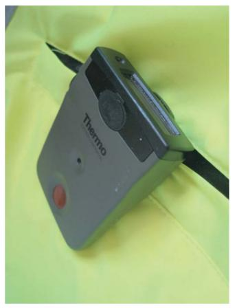
Figure 3.10 Electronic personal dosimeter.
