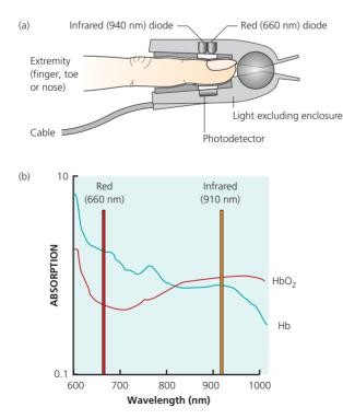
Figure 11.3 Pulse oximetry.
