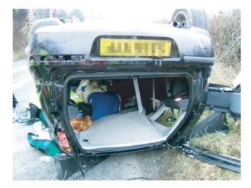
Figure 21.6 Access through rear hatch.
