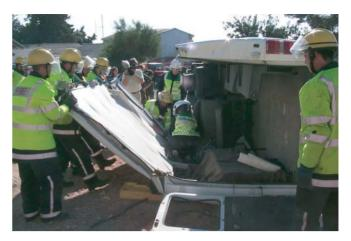
Figure 21.5 Roof fold-down.
