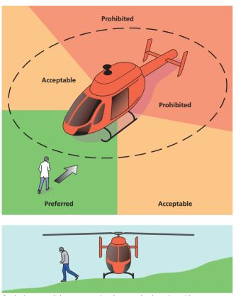
On sloping ground always approach or leave on the downslope side for maximum rotor clearance
