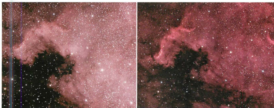
▲ A cooled CCD image of NGC 7000 (left) compared to a 10-minute exposure from a DSLR which was not cooled (right).
