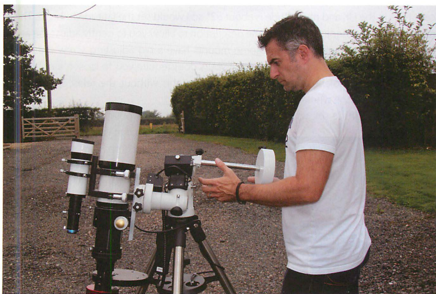
▲ Correctly balancing a telescope mount is vitally important. Mounts like this modern version of a German equatorial mount are balanced in both axes by first placing the declination axis horizontal.
