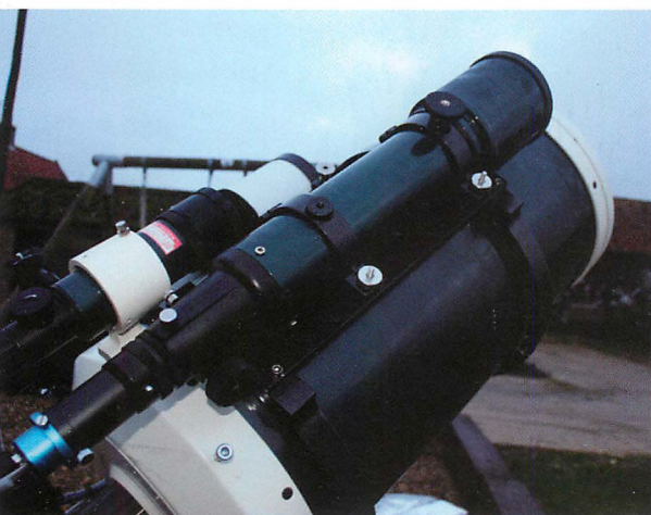
◀ Guide scope (80 mm refractor) and guide camera (QHY5-II) attached to the top of the author's telescope.
