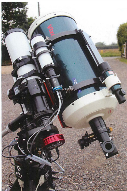
◀ The author's full imaging system showing the two imaging telescopes – 260 mm aperture (green) and 80 mm aperture (white) – with the guiding telescope on top. They are on a German equatorial mount.
