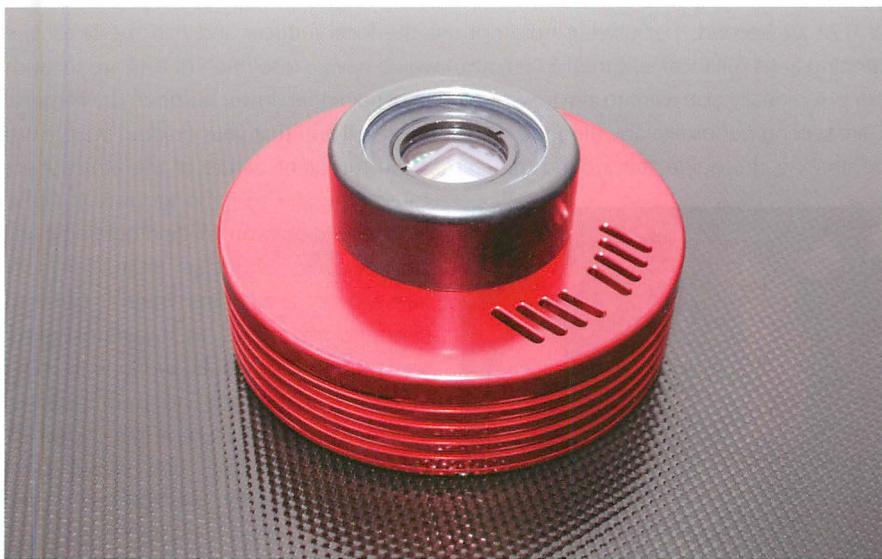
▲ The author's Atik 314L+ CCD camera, which was used for most of the deep-sky images in this book. It has a CCD chip measuring 8.9 \times 7.6 mm, with pixels just 6.4 microns across.
